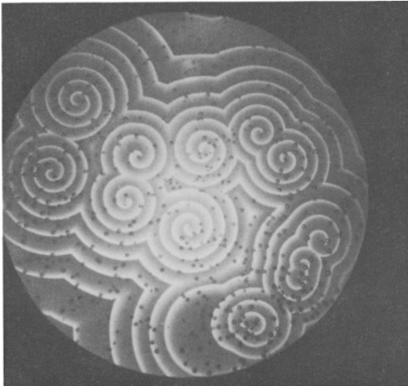
Fig. 1.20 a and b. Spirals of chemical activity in a shallow dish. Wherever two waves collide head on, both vanish. Photographs taken by A. T. Winfree with Polaroid Sx · 70.
