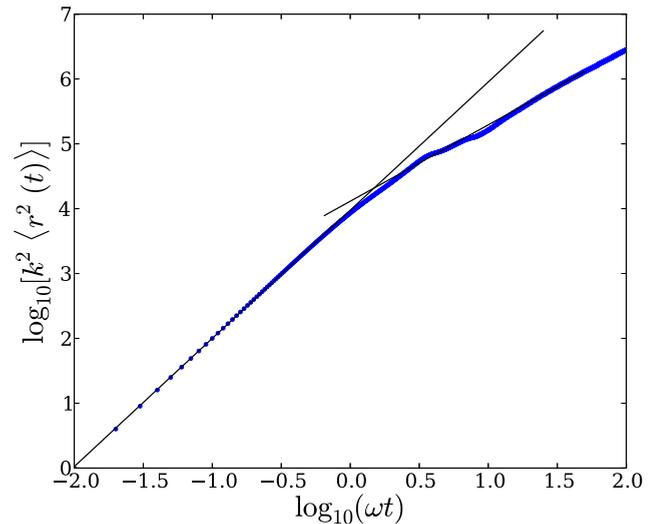
FIG. 1. (Color online) Average displacement  $\langle r^2 \rangle$  as a function of time for particles in a stationary ABC magnetic field ( $\omega = 0$ ). The ordinate is normalized with  $k^2$ . The two straight lines to the left and right of the curve are fits with slopes 1.9 and 1.1, respectively.
