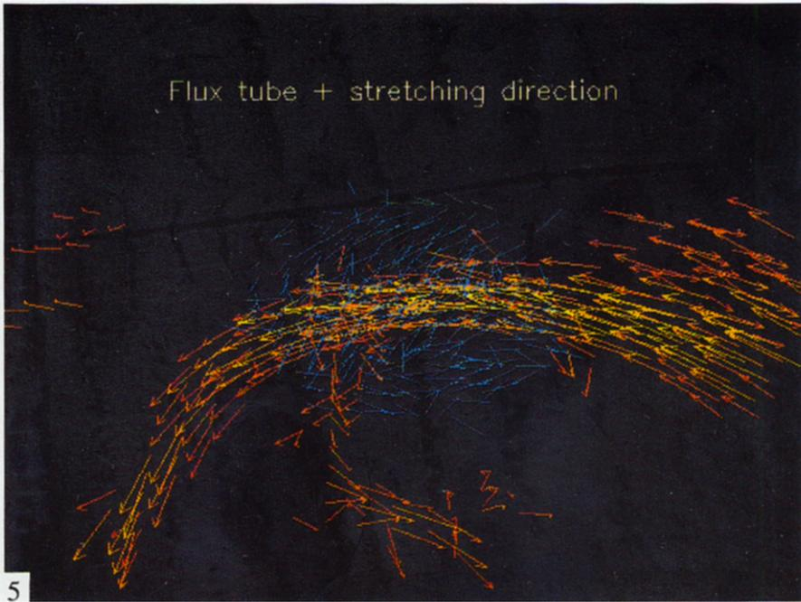
Fig. 5. Flux tube (from red to yellow as field increases) together with the eigenvector  $e_3$  (blue), corresponding to the direction of stretching, in a ball with a radius of 4 mesh points around the point of maximum magnetic field strength.
