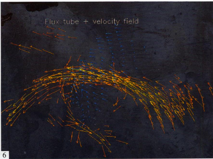
Fig. 6. Flux tube (from red to yellow as field increases) together with the actual velocity field (blue) in the plane perpendicular to the tube. Note that  $u$  tends to be aligned with the tube.
